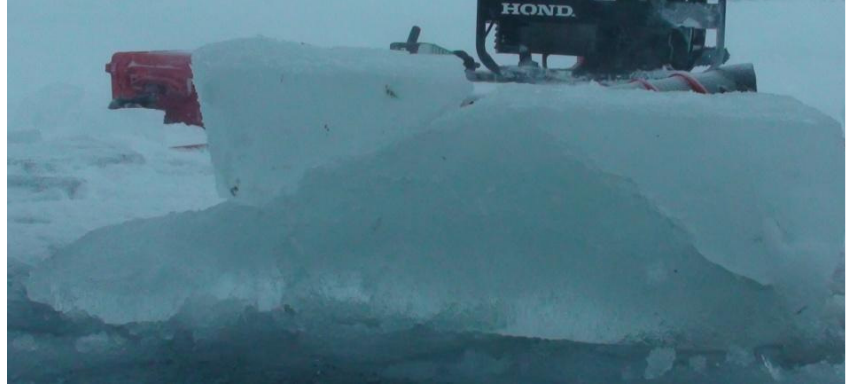
Photo 1. Punching in the fixed-ends beam test (short beam)
