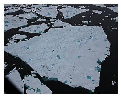
Figure 5. An extreme ice feature seen noted on a heli-recce. This is a small-medium (220m) size first-year floe with embedded heavy ridge elements having keel drafts estimated to be in excess of 15m. This ice feature would be a major challenge if encountered along a seismic line.
