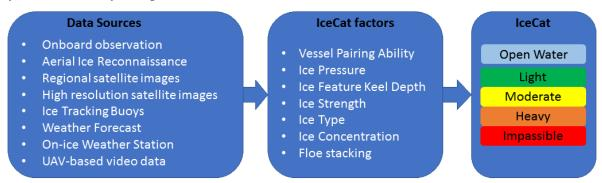
Figure 9. The data flow from input sources to factors considered in making an IceCat 1-2-3 chart to finally determine the appropriate color coding for the area of ice being investigated.
