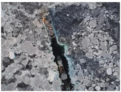
Figure 3. (2014) From 400m above, Fennica clearing the way for Shatskiy through light ice conditions. Note the clear wake aft of Fennica created by her powerful azimuth thrusters.
