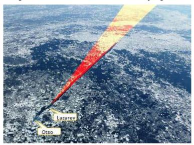
Figure 4. Otso (icebreaker) leads Lazarev (seismic vessel) through mixed ice conditions in NE Greenland. The black line shows the track that has been travelled while the red/yellow shading shows the potential offset of the seismic streamer should currents displace (in this concept example) the streamer to the right of track.
