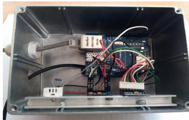
Figure 2. Photography of measuring sensor of automated system for control of planned position
