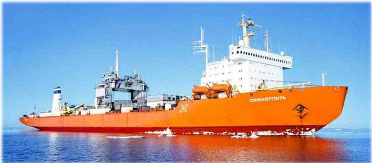
Figure 3. Nuclear powered ice-breaker LASH ship “Sevmorput”
