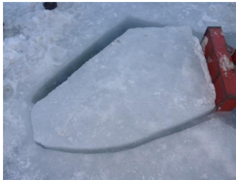
Figure 10. View of trapezium ("wide") specimen after testing.
