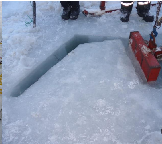
Loading of trapezium ("wide") specimen
