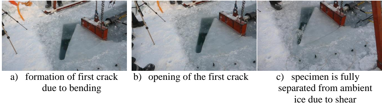
Figure 9. Testing of triangle ("narrow") specimen
