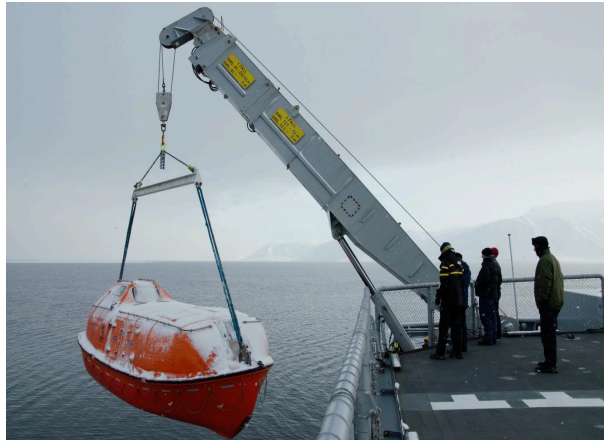
Figure 2. Lifeboat being lowered into the water with the deck crane. Photo © Jan Erik Jensen
