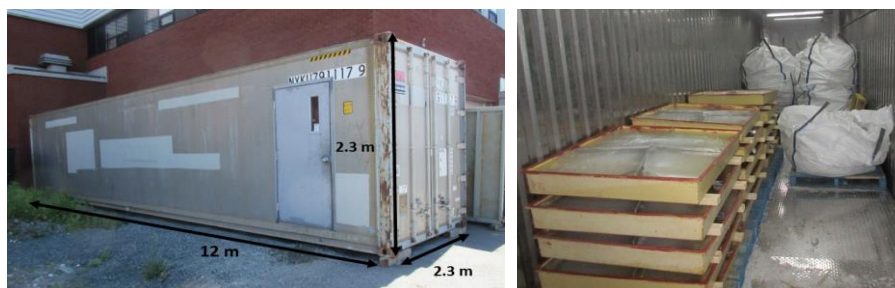
Figure 4. Ice rubble production and storage inside the refrigerated container
