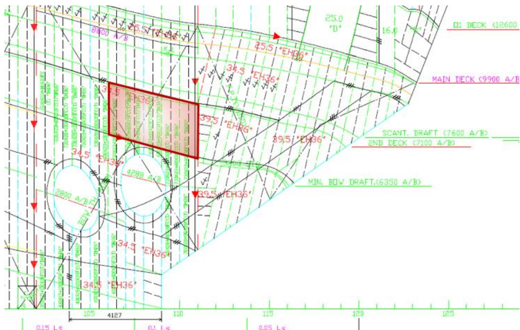
Figure 2. Area instrumented by strain gauges in the IBRV ARAON (Kim, 2014) POAC17-108
