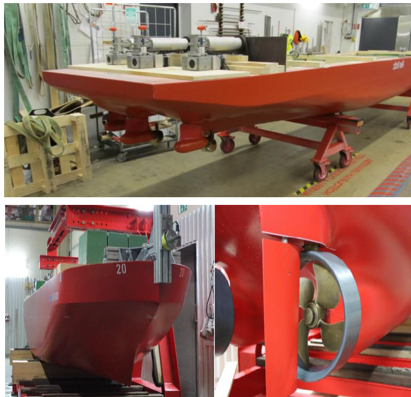
Figure 4. Stern of the model ships (Pod-driven ship: Top, Twin-screw ship: Bottom)
