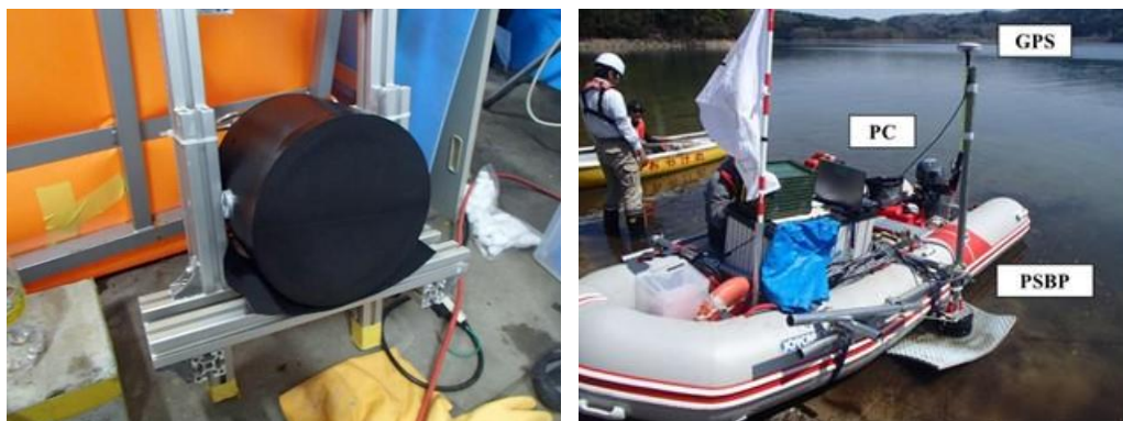
Figure 7. Sensor probe of PSBP (left) and experimental setup (right)
