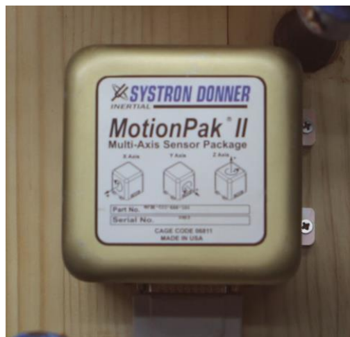
Figure 1. Inertial measurement system “MotionPak II” of SYSTRON DONNER INERTIAL, Inc.,
