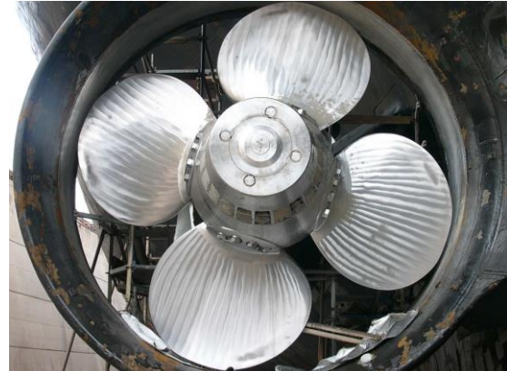
Figure 5. The FS Polarstern has a ducted propeller design.
