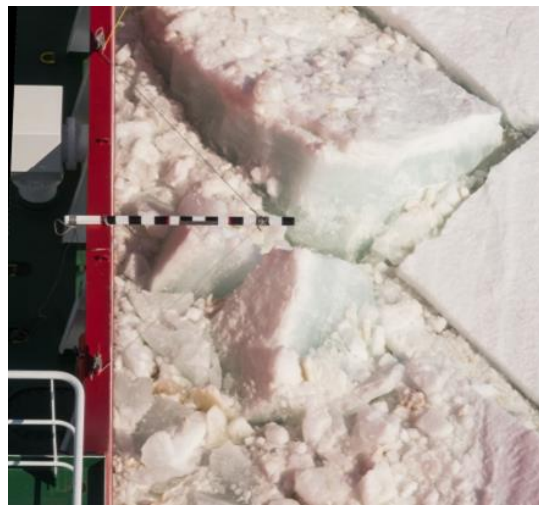
Figure 2. The measurement stick for ice thickness estimation. Each stripe is 10 cm wide.
