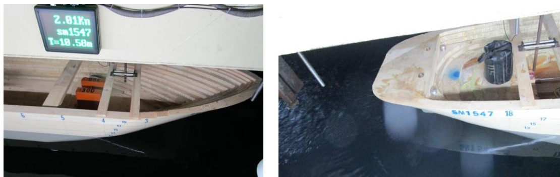
Figure 4. The towing test at speed of 2kn
