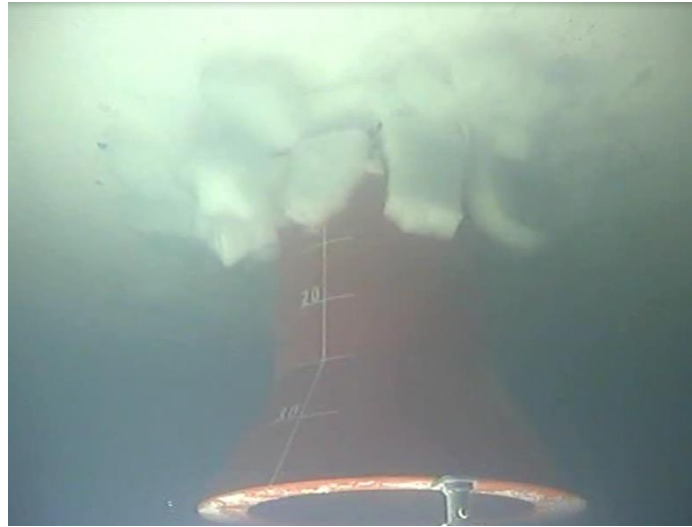
Figure 12. Ice rubble accumulates near the structure, beneath the ice, still from model test video (HSVA 2010a)
