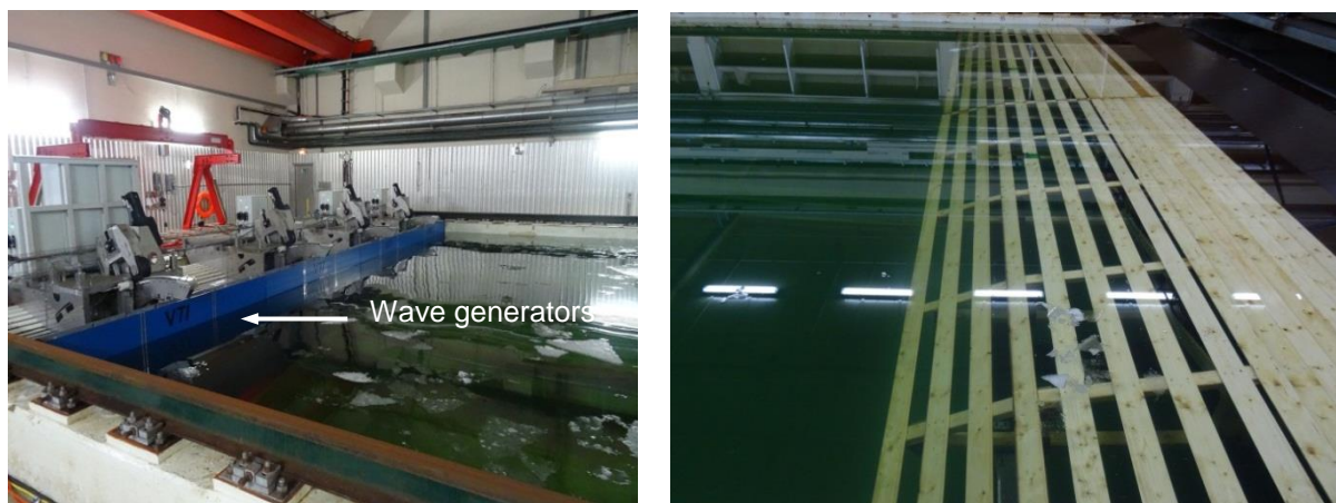
Figure 2. Mobile wave generator modules (left) and parabolic shaped beach (right).
