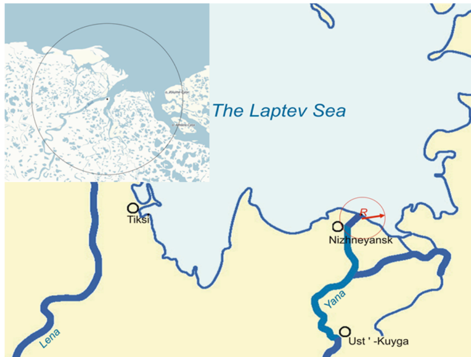
Figure 1. Estimated range of the coverage area of base station (BS) of Automatic identification system (AIS) in the estuary of the Yana River
