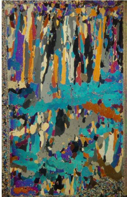
Figure 3. Thin section of the ice showing the initial vertical columnar structure that became disrupted and somewhat jumbled (about half-way down the image). The markings on the
