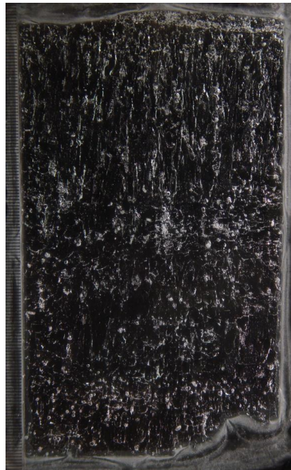
Figure 4. Same thin section as in Figure 3., with side lighting and without using polaroid filters, showing brine and air filled channels and pockets in the ice. The section is 1.0 mm thick. The markings on the scale at the left are mm scale at the right are mm. The section is 0.5 mm thick.
