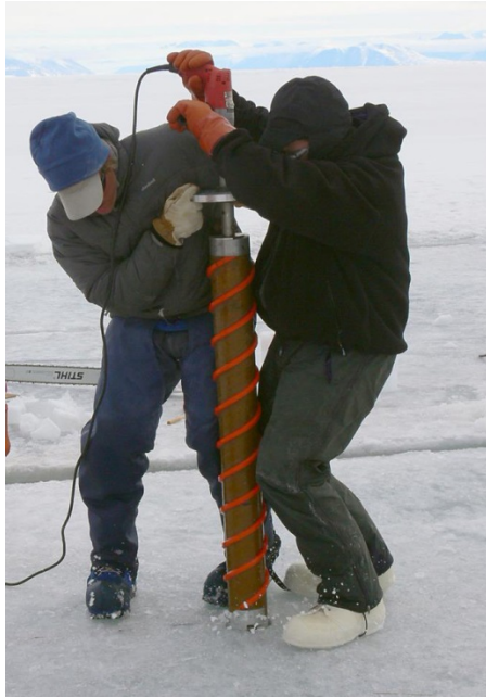
Figure 7. Coring with a drill: disk that stops the corer plunging down is visible.
