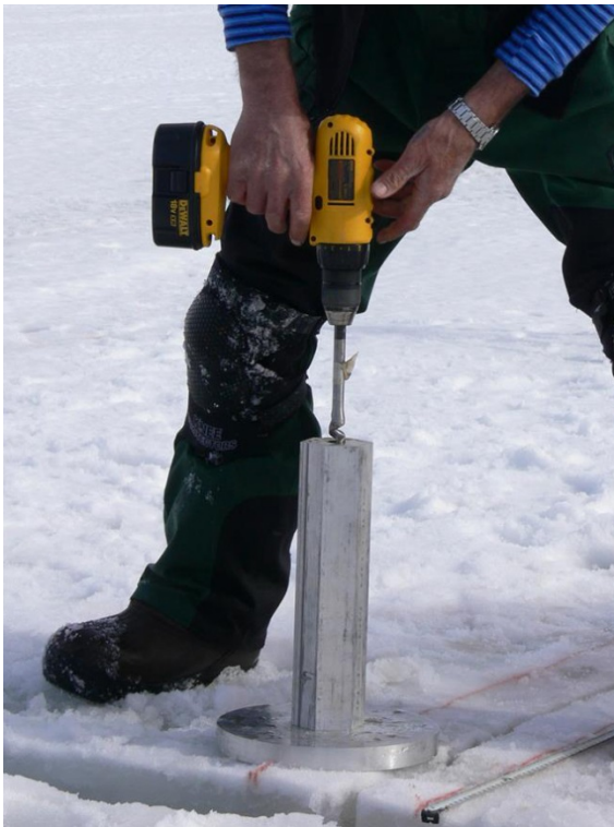
Figure 6. The drill chuck used to drill holes for the dowels.
