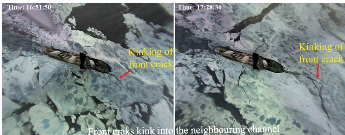
Figure 4. Repetitive observations of front crack kinking into the closest channel on August 28 th , 2013.
