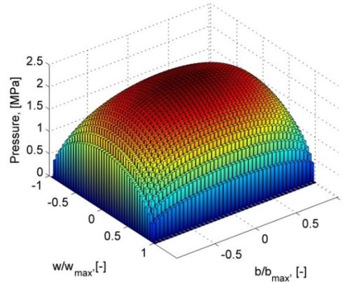
Figure 3. An example of spatial pressure distribution that was calculated with the Kurdyumov and Kheisin model.
