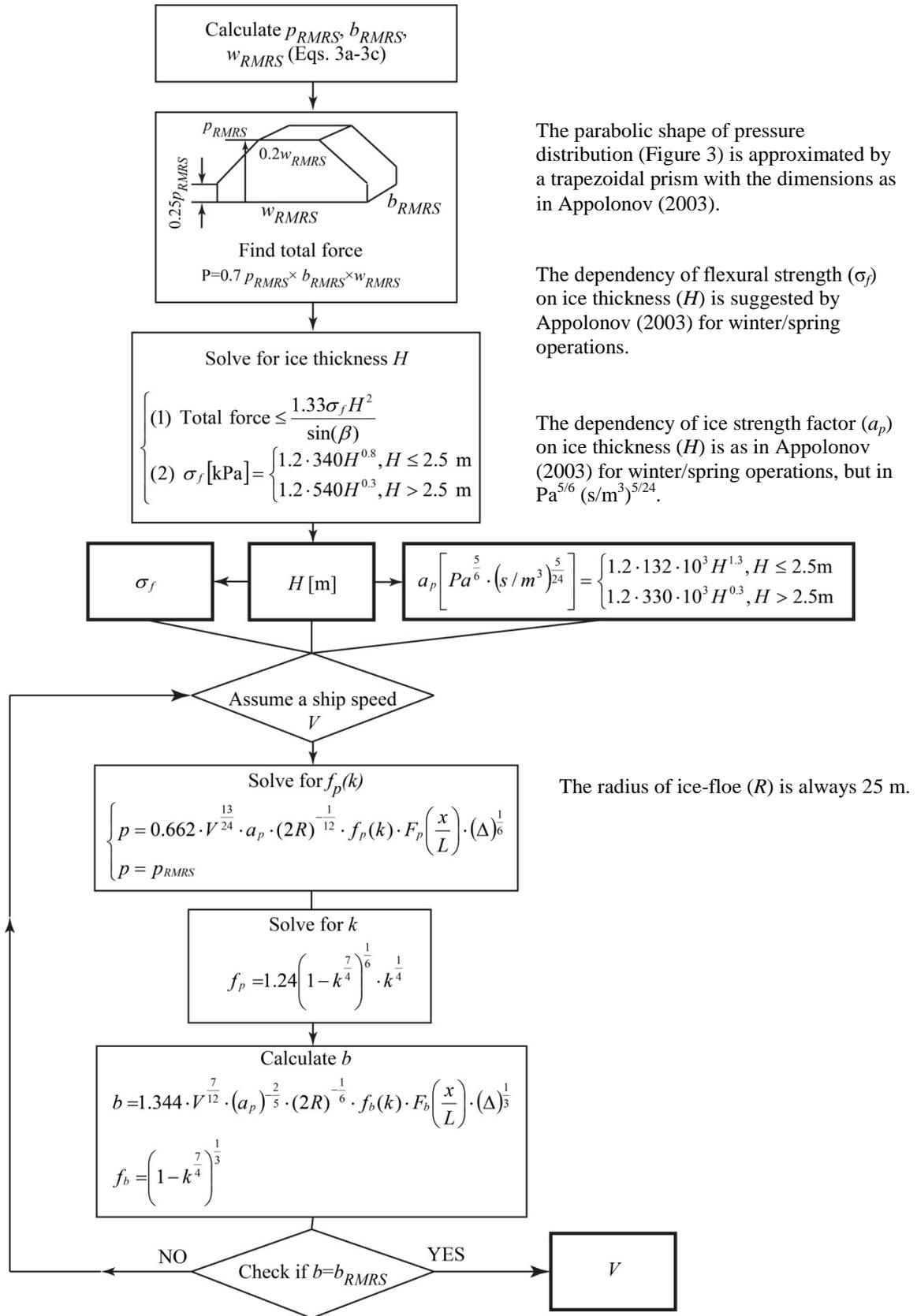
Figure 4. A workflow diagram that shows how to determine physical parameters such as flexural strength, ice thickness and ship's speed before the impact from the known ice class factors.
