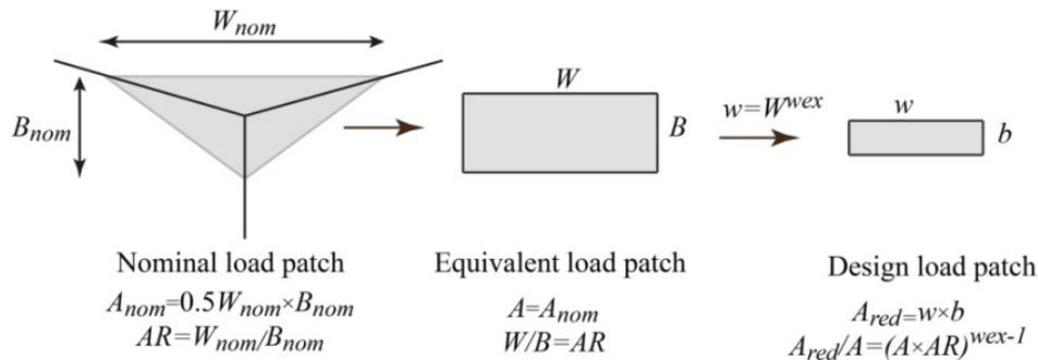
Figure 2. Nominal, equivalent and design load patches.
