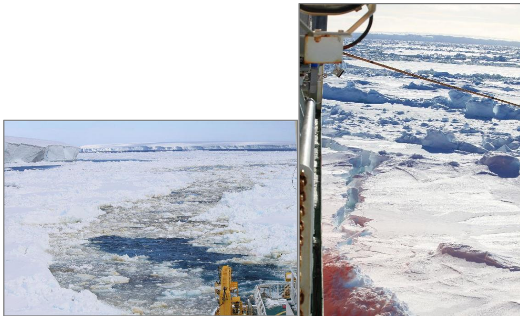
Figure 3. General ice transit and repeated ramming mode under heavy ice condition
