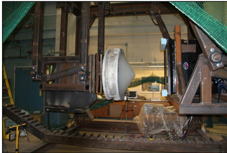
Figure 1: Large pendulum apparatus with ice cone mounted on the left carriage and Impact Module on the right.
