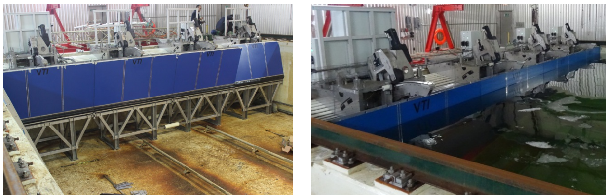
Figure 8. New flap type wave generator in HSVA's large ice model basin consisting of four removable units
