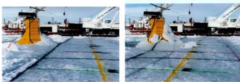
Figure 2. Intermediate-scale test on sloping-sided structure in the Esso basin. (Metge, M. and Tucker, J.R., 1990; with permission of Imperial Oil, Calgary)
