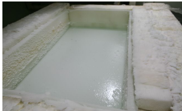
Fig. 8 The granular EG/AD model ice with good visibility
