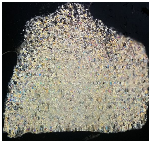
Fig. 6 Cross section of granular EG/AD model ice (about 35 mm)
