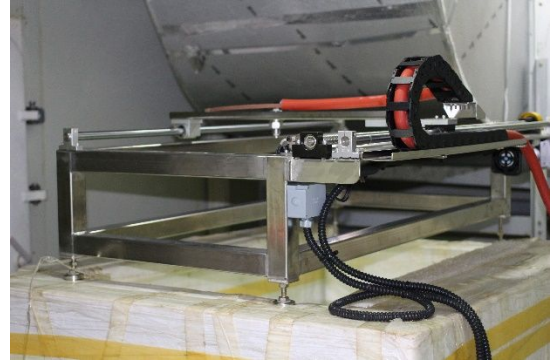
(b) Auto-spraying machine with the miniature tank
