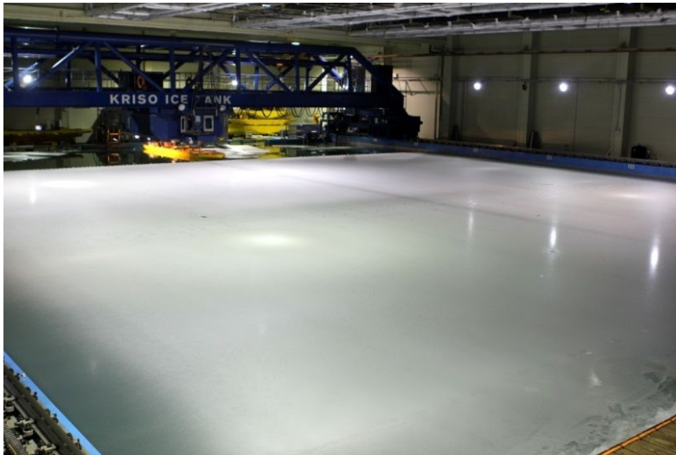
Figure 1 Generated EG/AD-CD model ice in KRISO ice tank
