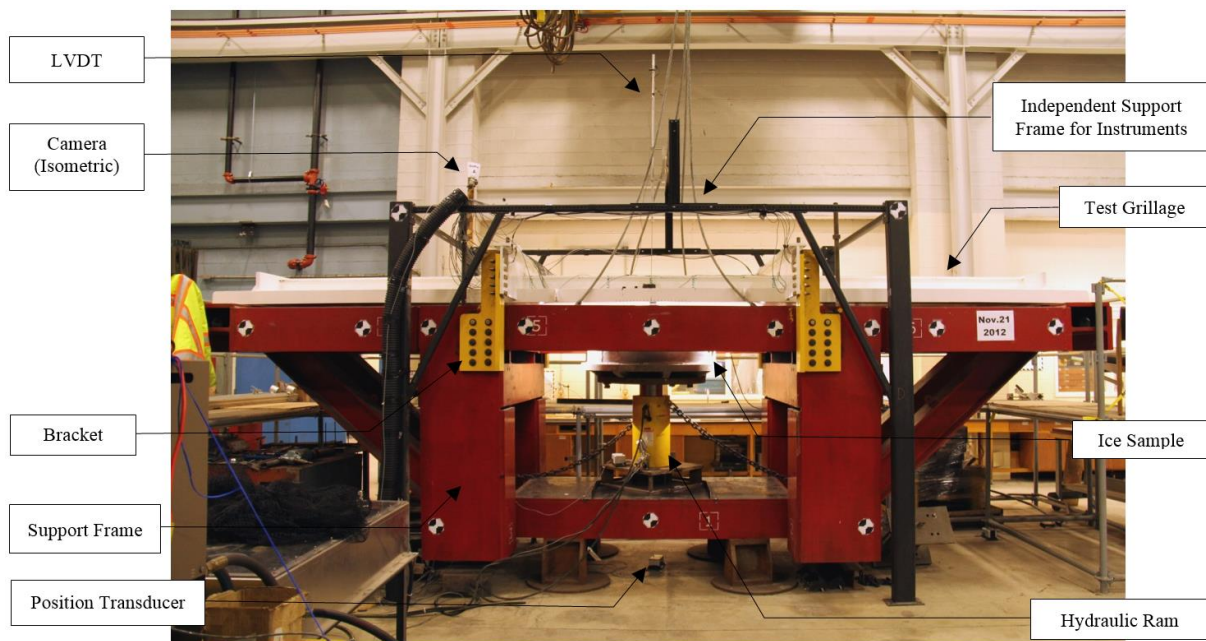
Figure 1. Grillage test apparatus
