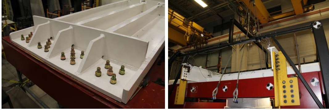
Figure 3. Boundary conditions at the longitudinal ends(left) and at the stringer ends(right)
