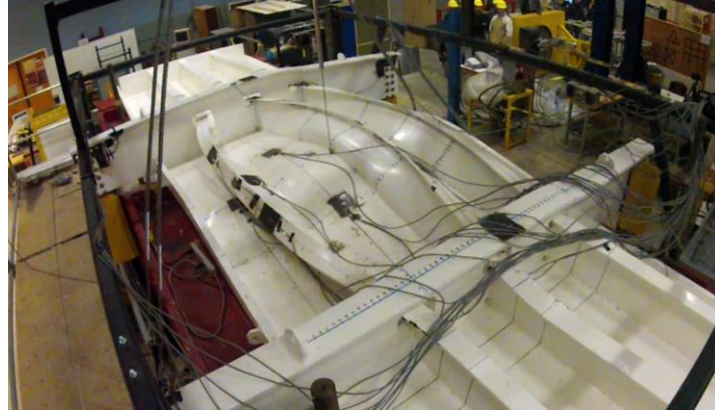
Figure 6. Isometric view of Grillage #1 at maximum load (2.8 MN)
