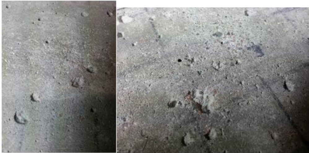
Figure 9 Concrete abrasion on the high performance concrete sample (left) and low performance concrete sample (right) over a test sequence. The location is at the starting point of the test runs as shown with the cross in Figure 3. The loading on the high performance concrete sample is much higher (Ice loading: W_n = 2.6 \text{ J/mm}^2 and W_s = 0.2 \text{ J/mm}^2 ) than for the low performance concrete sample (Ice loading: W_n = 1.25 \text{ J/mm}^2 and W_s = 0.5 \text{ J/mm}^2 ).
