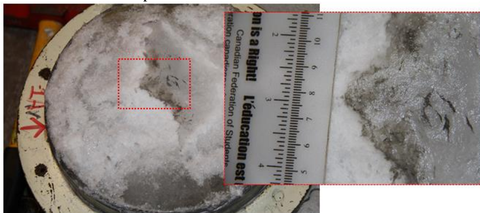
Figure 10 Concrete dust and particles enclosure under recrystallized ice after test 1a ( v_n = 1.0 \text{ mm/s} / v_s = 18.0 \text{ mm/s} ) at the high performance concrete sample
