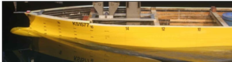
Figure 5. Photo of resistance test at 15 knots (ballast draft).
