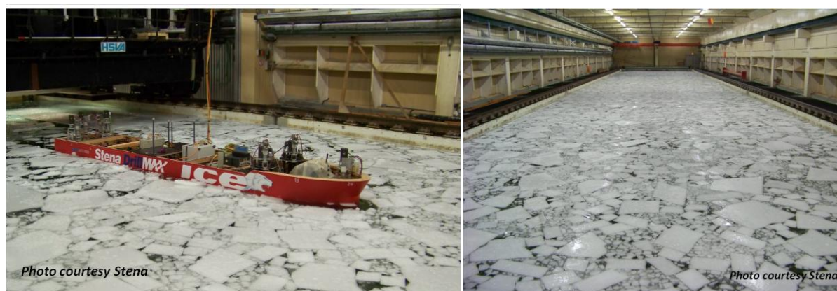
Figure 6. 2011 IceMAX DP Model Test in Full Scaled Based Managed Ice Conditions
