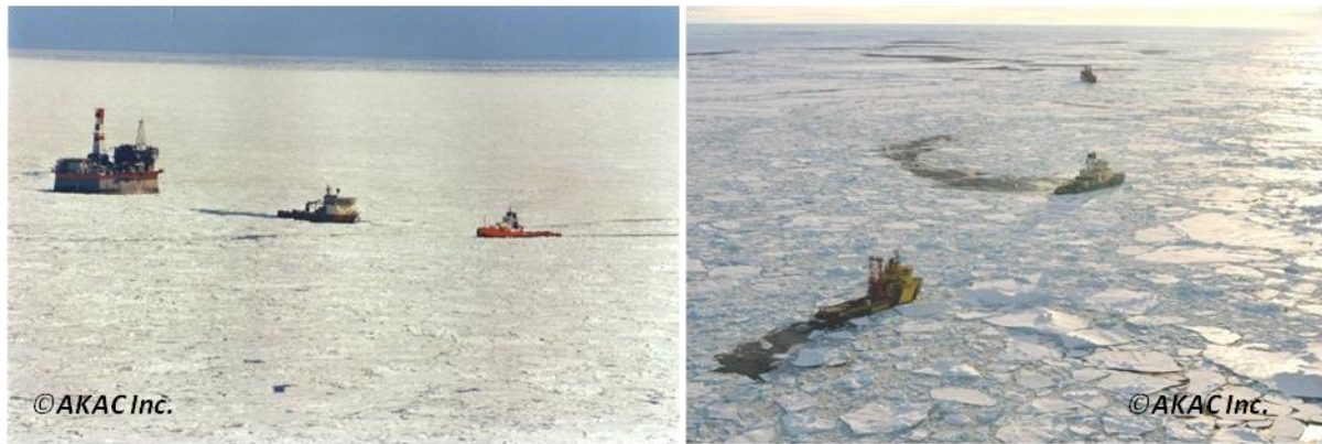
Figure 1. Previous DP operations performed in pack ice, CSO Constructor in Sakhalin (left) and Vidar Viking during ACEX (right), both supported by physical ice management.
