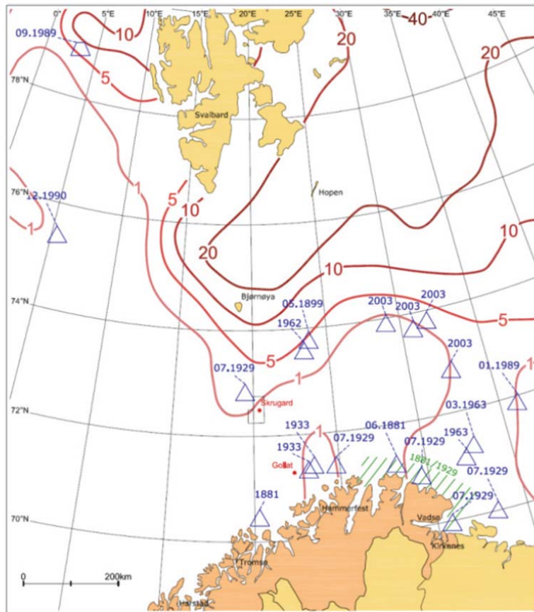
Figure 2. Iceberg occurrence in the Barents Sea. The contour lines are the annual probability (%) of occurrence of icebergs in a 100 x 100 km cell. Triangles and shaded areas are abnormal observations of icebergs. The map is prepared by Multiconsult based on figures in Abramov (1996).
