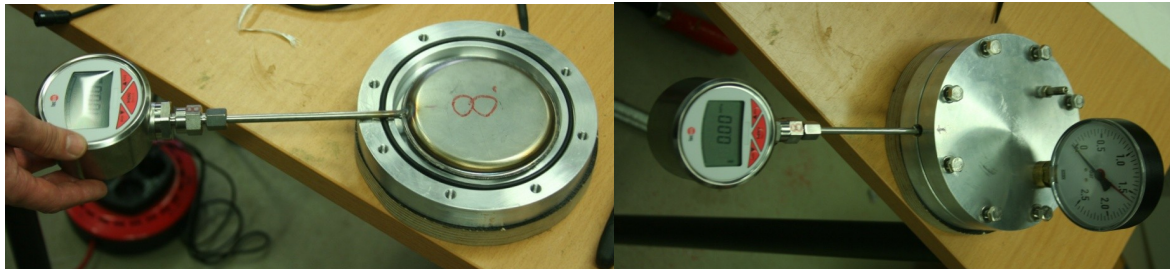
Figure 1. Calibration with air pressure. The device on the left and device ready for air pressure calibration on right.
