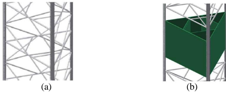
Figure 1 - (a) Open truss type leg; (b) shielded Jack-Up leg
