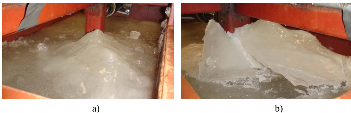
Figure 6. Indenter and ice before (a) and after (b) the experiment 4m in the second set of experiments.
