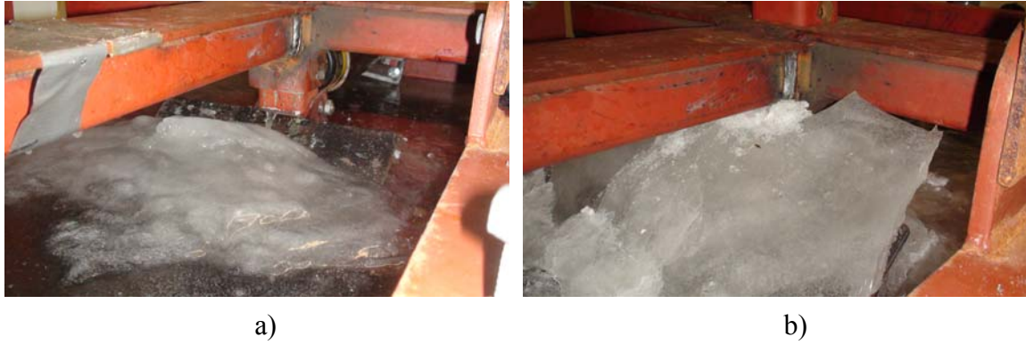
Figure 8. Indenter and ice before (a) and after (b) the experiment 2 of the third set.
