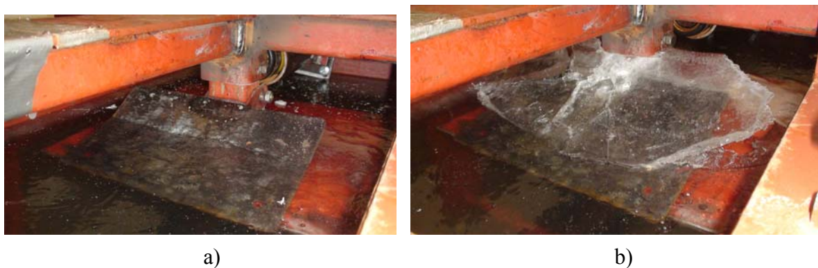
Figure 7. Indenter and ice before (a) and after (b) the experiment 1 of the third set.
