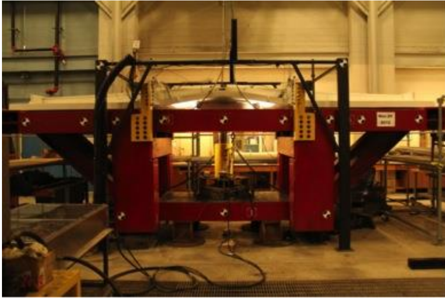
Figure 5: The grillage at maximum deflection during experimentation
