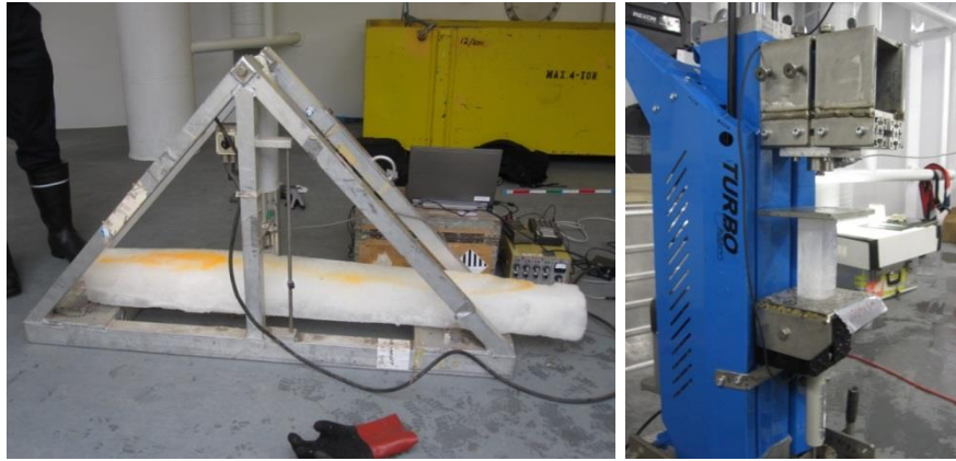
Figure 5. Test setup for obtaining ice flexural strength (left) and compressive strength (right) measurements.
