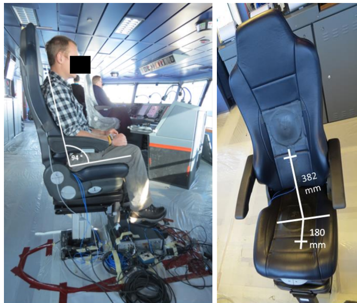
Figure 2. A seated occupant on the Cleeman seat on the bridge of the vessel (on the left) and the placement of the seat-pad accelerometers for whole-body vibration measurement (on the right).
