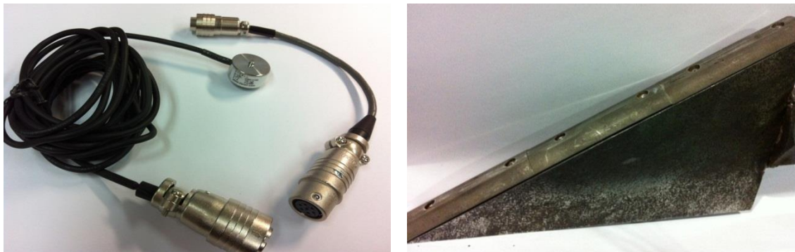
Figure 3. Equipment for the ice tests; Load cell (left) and jig of triangle shape (right).
