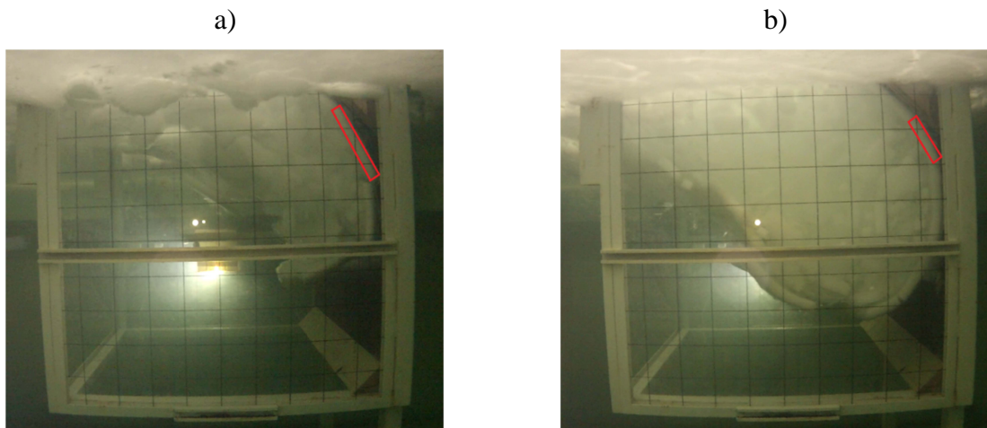
Figure 3. Decreasing block size during the interactions, here test run 5210, in a) a large beginning of interaction level ice block is highlighted; in b) a large end of interaction ice block is highlighted.
