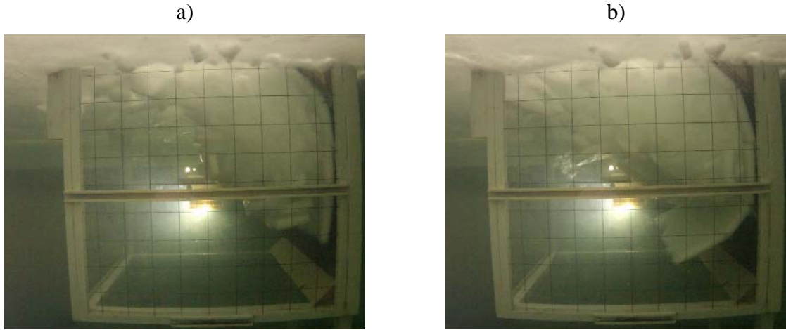
Figure 5. Collapse event during test run 5210, 120 s; in a) the rubble reaches a maximum depth; in b) the rubble has just collapsed and extends further away from the inclined panel.
