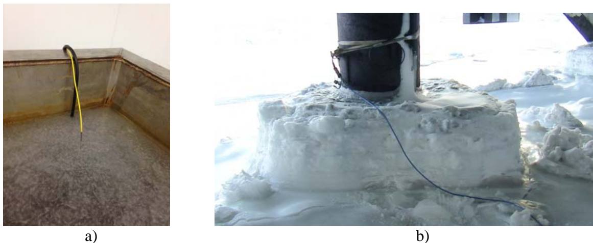
Figure 3. FBG and EBA thermistor strings in the ice tank (a) and in the ice bustle (b).
