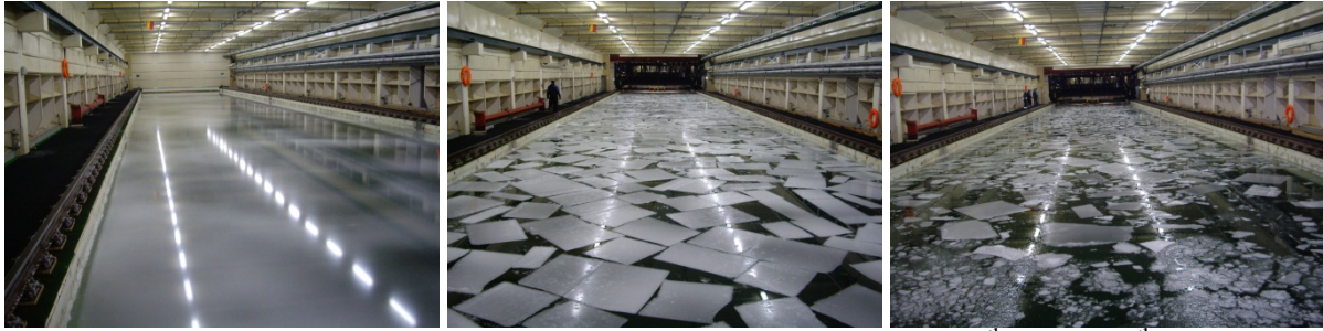
Figure 1. Ice concentrations in the ice tank: level ice, 8/10 th and 6/10 th .
