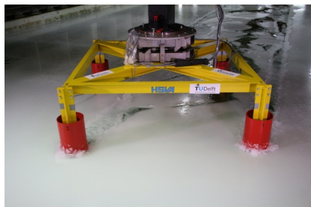
Figure 2. a) Dimensions of the jack-up in full scale and in model scale. b) The jack-up model at 22.5° orientation in level ice.
