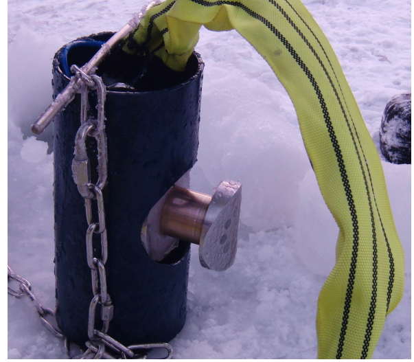
Figure 2. The UNIS-BHJ with piston fully extracted at 50 mm.
