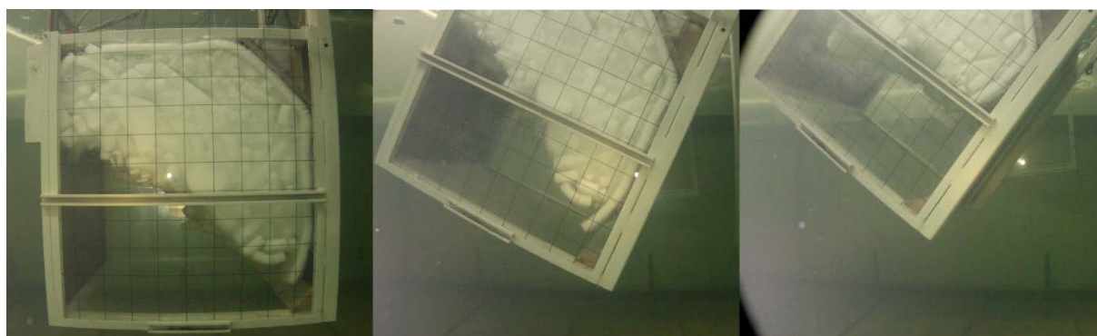
Figure 4 Submerged stability test 3230 at different inclination angles: 0°; 25°; 39°
