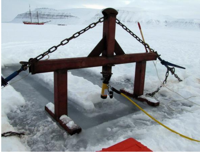
Figure 5. Experimental set-up before the bending tests (left) and an example of the force record (right)
