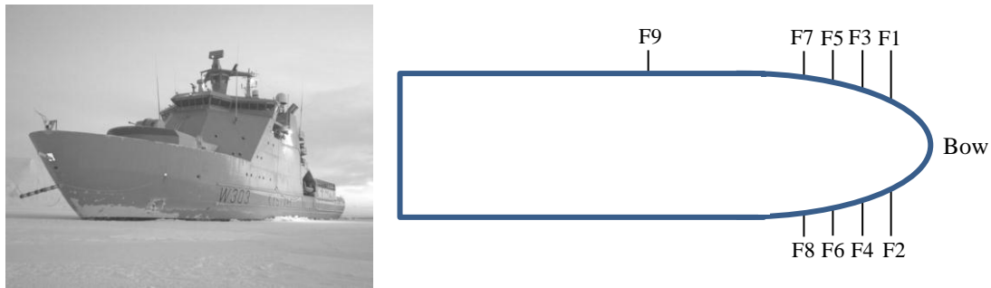
Figure 1 Photo of KV Svalbard and plan view of the locations of strain sensors
