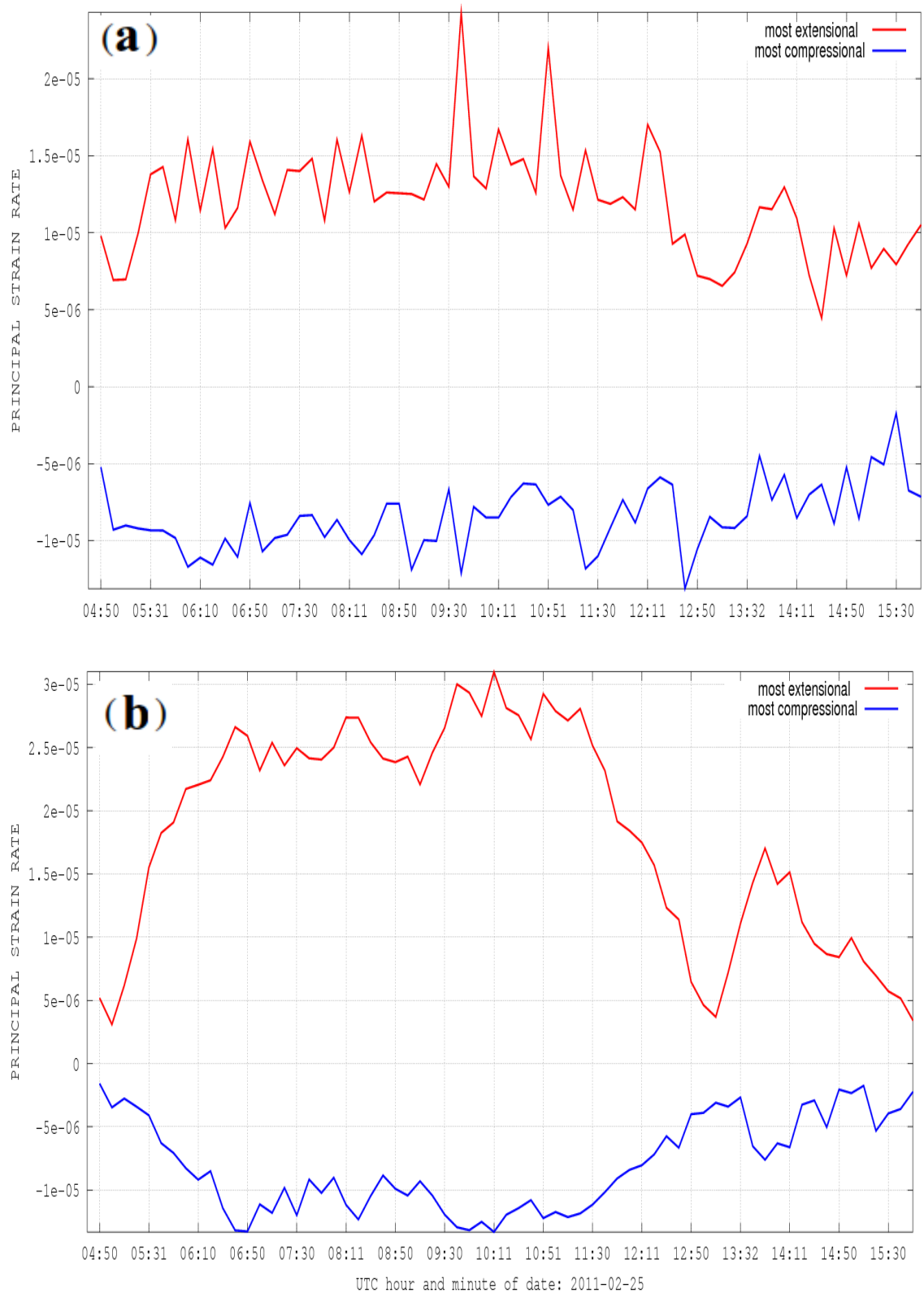
Figure 4. Example of mean principal strains computed on based virtual buoys for the Feb 25, 2011 case, \epsilon_1 as red and \epsilon_2 as blue. The time step is 10 min.
