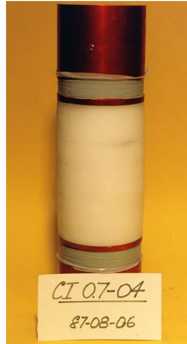
Figure 3. Ultimate Stress vs. Confining Stress and Sample after T451
