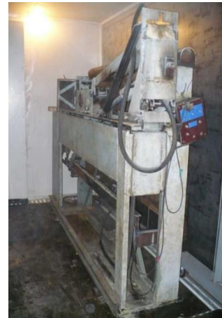
Figure 10. The testing on the ice abrasion Hydrotex Co. Ltd
