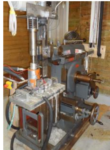
Figure 9. The testing on the ice abrasion NTNU (COIN, 2008)
