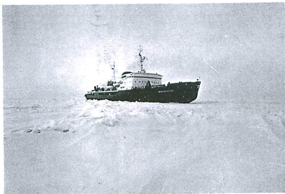
Fig. 10. VLADIVOSTOK, a polar icebreaker of Moskva type, in ice trial.
