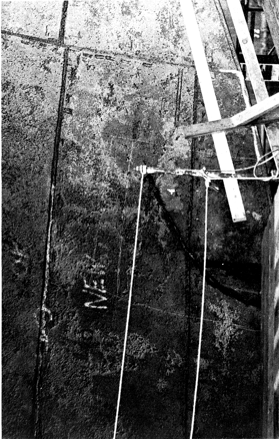
Figure 1: A and B strakes, starboard bow, USCGC NORTHWIND, November 1967. Although intended to show ice damage, this photograph illustrates well the extensive pitting of the shell plate, the corrosion of the original welds, and the concentrated attack in heat-affected zones caused by flame cutting the builder's clips and brackets.
